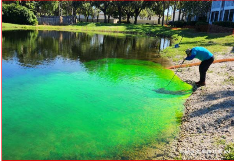
Photo N5— Leaking dye observation.
