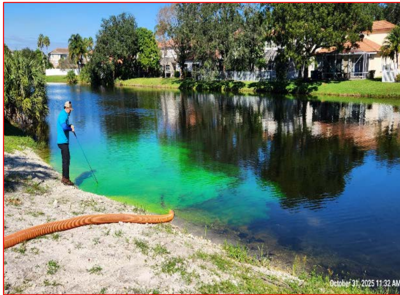
Photo N6— Prove pipe location.
